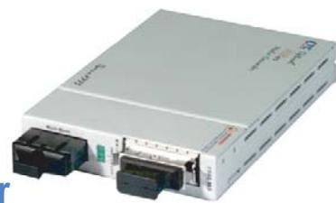
The FIB1-1000MG is a multimode (850nm) to single mode (GBIC module) fiber optical media converter and repeater that allows data rates up to 1.25Gbps. The converter performs re-amplification and re-shaping of the optical signal. This converter is compatible with fiber interfaces such as FDDI, STM-1, STM-4, OC1, OC3, OC12, OC24, 1G fiber channel, fast and Giga Ethernet.
