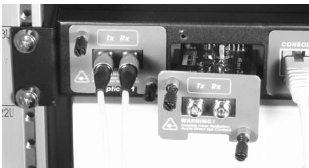
Pull out the module by the captive screws.
